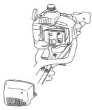
Some mufflers are equipped with a special spark arrestor screen. If your machine has this type of muffler, you should clean the screen at least once a week. This is best done with a wire brush.
